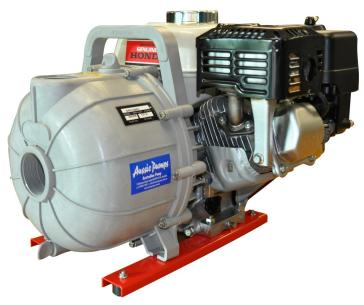
Aussie polypropylene 2" self priming centrifugal chemical pumps offer flows to 835 litres per minute and heads as high as 25 metres. Suction lift is 7.6 metres.
